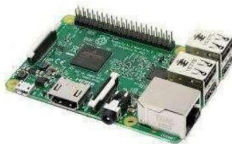
Gambar 3. Raspberry Pi 3 B
